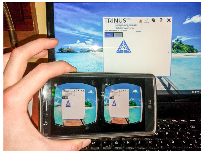
Figure 2: TrinusVR streaming the computer desktop to a mobile phone to be used in Google Cardboard.
