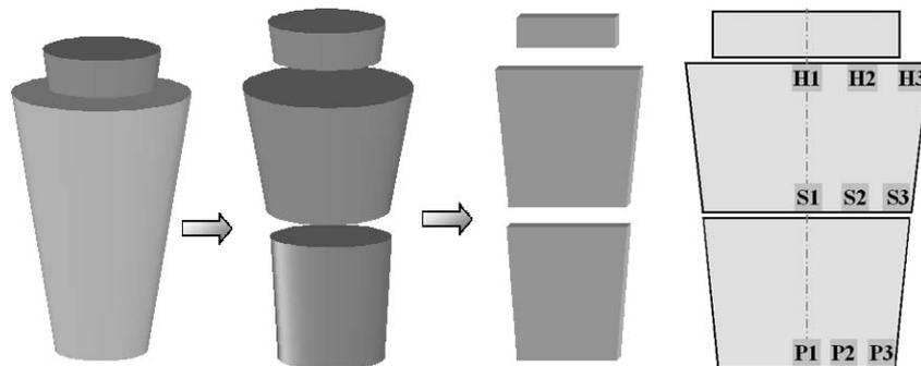
**Figure 5:** Steel ingot dividing and sampling diagram
