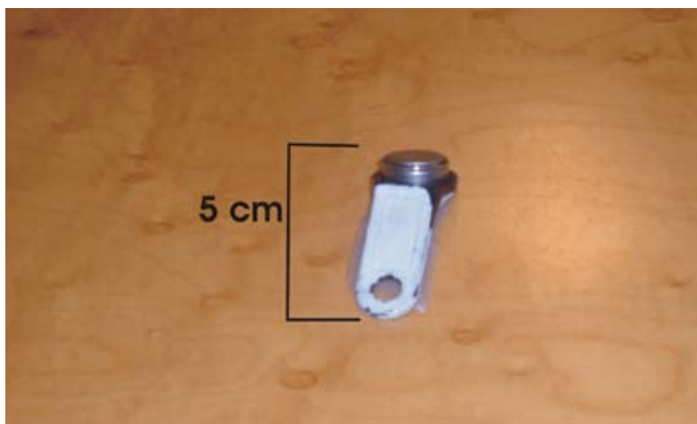
Figure 3: A digital thermometer, known also as i-button on a white clip (Photo: M. Ogrin).
