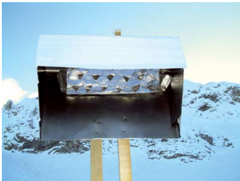
Figure 2: A radiation shield for an alcohol thermometer (Photo: M. Ogrin).
