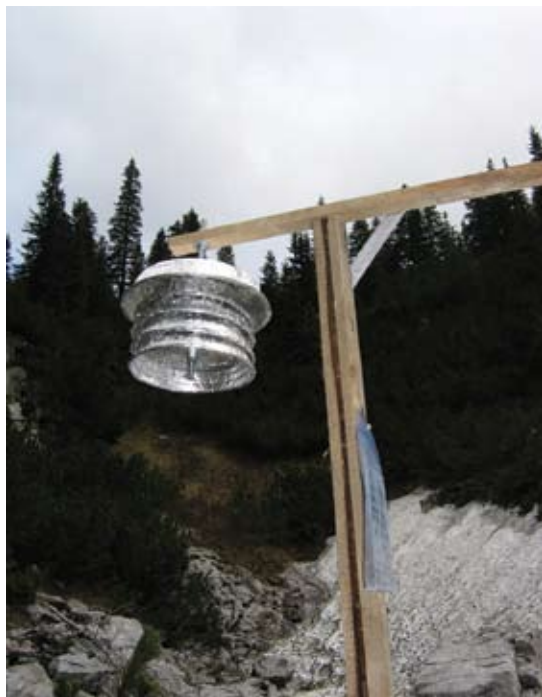
Figure 1: A radiation shield for a digital thermometer (Photo: I. Sinjur).
