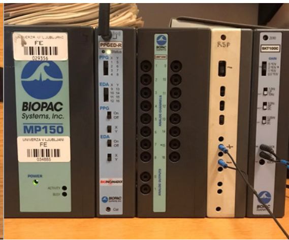
Fig. 5: Electrodermal activity sensor with wet electrodes (left) and MP150 Biopac Systems device (right)
