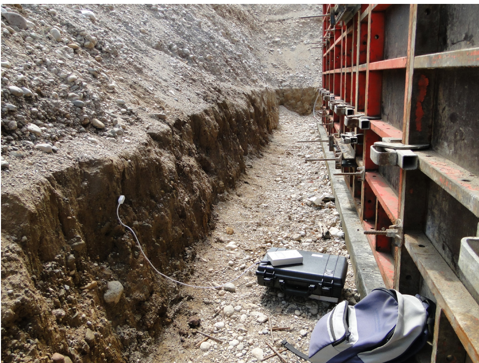
Fig. 4. Field measurement of the thermal parameters with the KD2 Pro meter.
