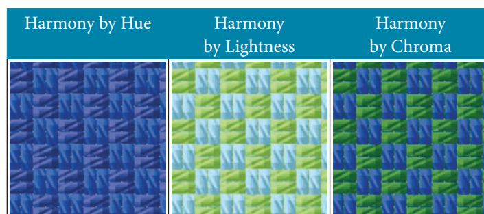
Figure 28: Merging effect of colours being harmonic by hue and lightness (Picture was made by using CAD program by Arahne [22].)
