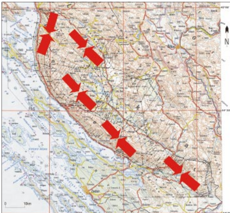
Fig. 7: Strain trajectories with maximal stress orientations indicated with arrows.
