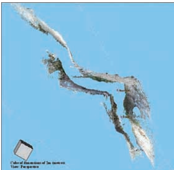
Fig. 5: Presentation of a combined (joint) scan; Kraški rob wall on the right and the wall with the Črni kal castle on the left.
