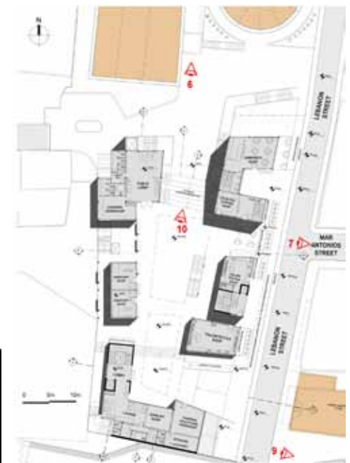
Figure 4: Ground floor plan showing the different shops, workshops, in relation with the street, the main piazza, and the heritage buildings (in brown).
