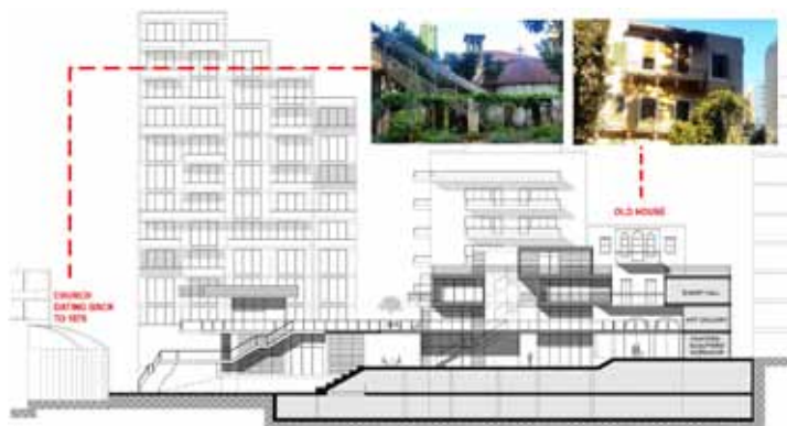
Figure 5: Longitudinal section D cutting through the main piazza linking the two heritage buildings (the church and the old house), and showing the interior series of shops
