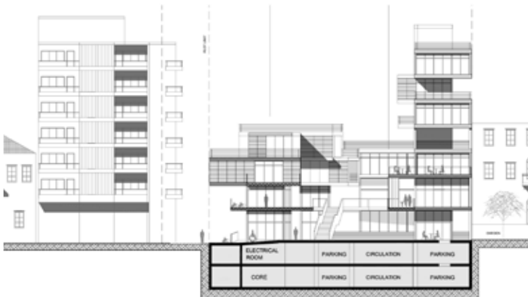
Figure 8: Section cutting through Mar Antonios Street and showing the existing street façade piercing into the project.
