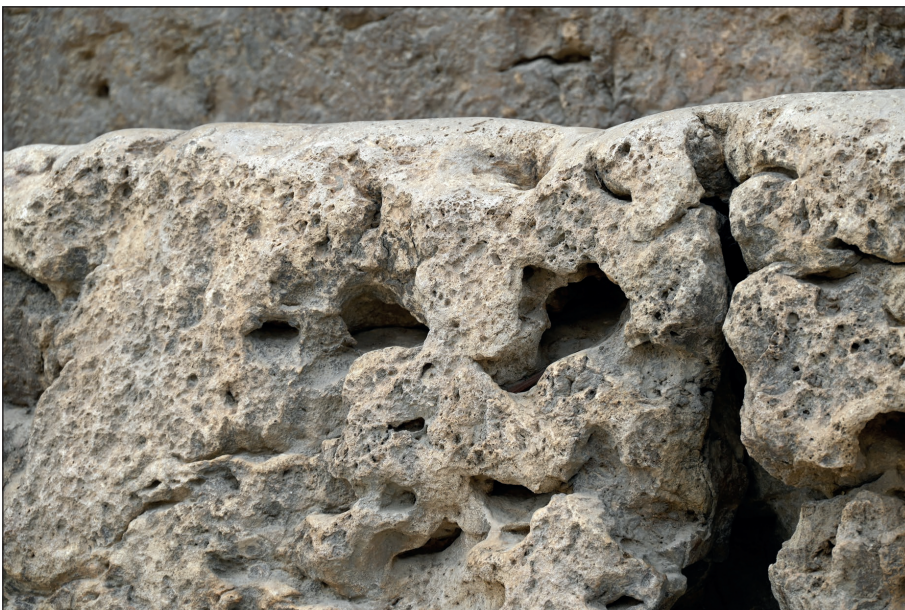
Figure 3: Hollowness of the bedrock limestone. Width of view is 2 m.
