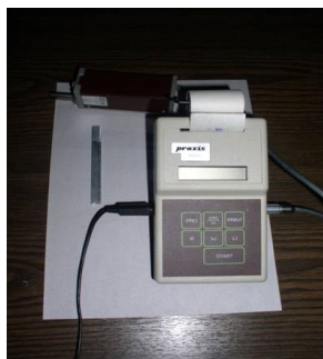
Fig. 4. The equipment for surface roughness measurement
