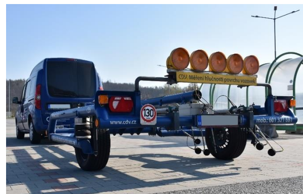
Figure 1: Open CPX trailer designed by Transport Research Centre.
