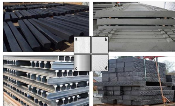
Figure 3: Different types of railway sleepers; wooden railway sleeper (a), concrete railway sleeper (b), steel railway sleeper and composite railway sleeper (d).
