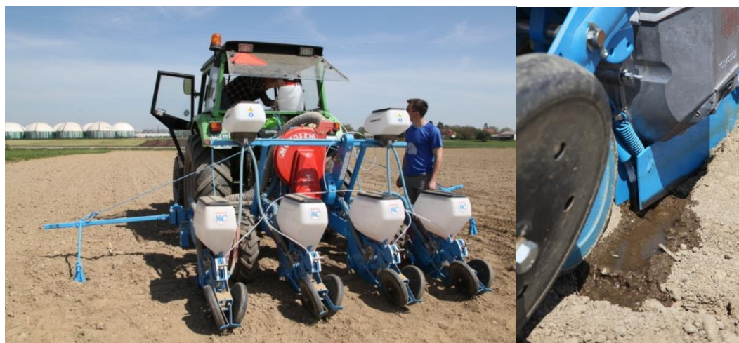
Figure 1: (A, B) Nematodes were applied to the field plots during sowing of maize as a fluid stream into the seed furrows, at a depth of 8-10 cm
