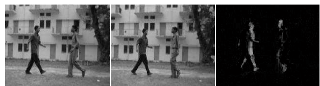
Figure 4: Example of object detection using temporal differencing technique
