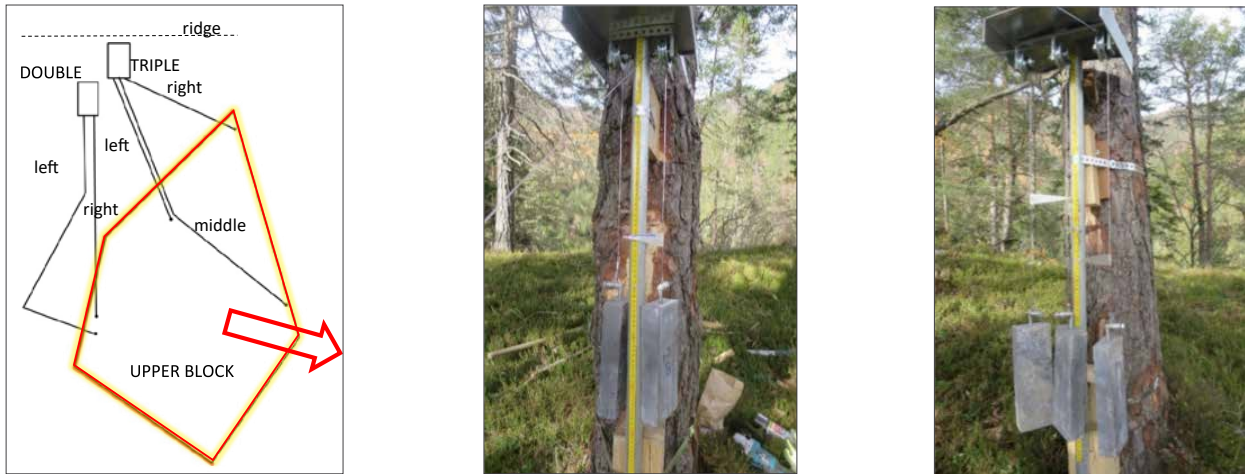
Figure 3. Left: schematic position of the wire extensometers, based on the upper block and based on the potential direction of movement; Right: a double and triple extensometer.
