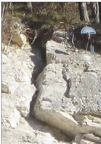
Figure 5. Left: view of the extensometer in September 2015; Middle: view of the extensometer in June 2016; Right: view of the extensometer in May 2017. The difference is 11.0 mm. The increase of the value occurred between January and June 2016 (5 mm), as well as between November 2016 and May 2017 (6 mm).
