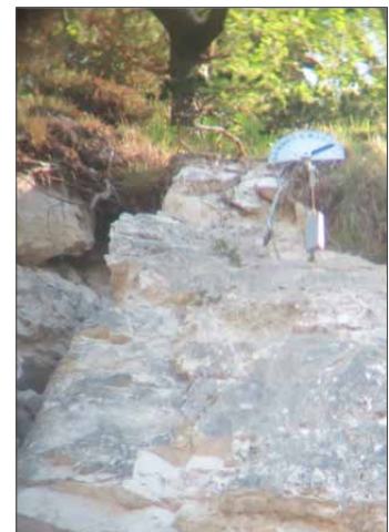
Figure 5. Left: view of the extensometer in September 2015; Middle: view of the extensometer in June 2016; Right: view of the extensometer in May 2017. The difference is 11.0 mm. The increase of the value occurred between January and June 2016 (5 mm), as well as between November 2016 and May 2017 (6 mm).
