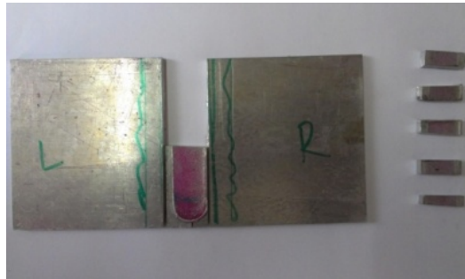
Fig. 3 Welded sample: A cut into pieces for corrosion testing
