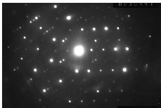
Figure 42: Diffraction from carbides of Figure 41, with double-diffraction effects
