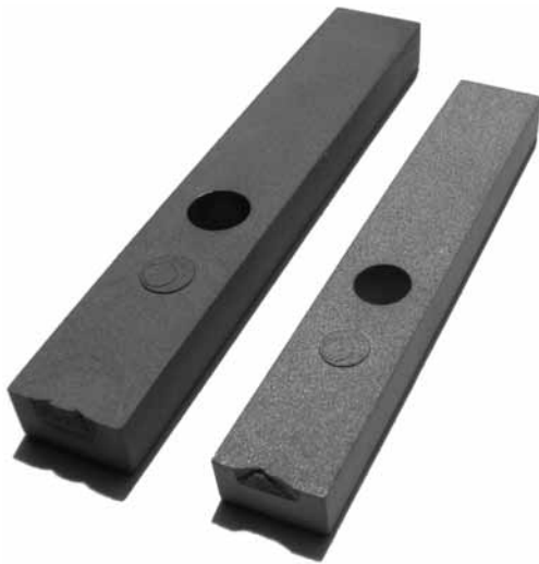
Figure 7: Green and sintered specimens used for the analyses Slika 7: Zeleni in sintrani kos, uporabljen za analizo
