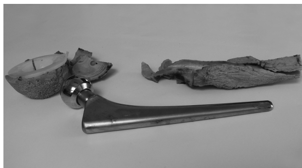
Figure 1: Hip prosthesis together with acetabular cup and residues of cement after being surgery removed
