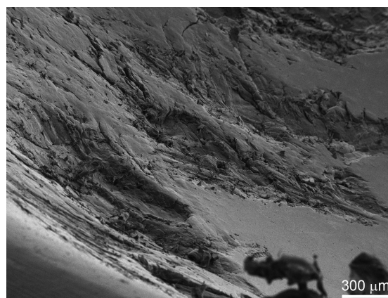
Figure 2: Surface modification of the polyethylene acetabular cup's inner wall with deep cavities, SE image
