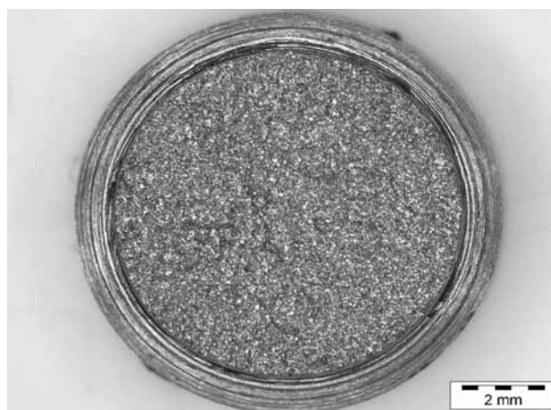
Figure 7: Fracture surface of a notched tensile specimen cooled in a lead bath from 1250 °C. Microstructure: coarse-grained bainite
