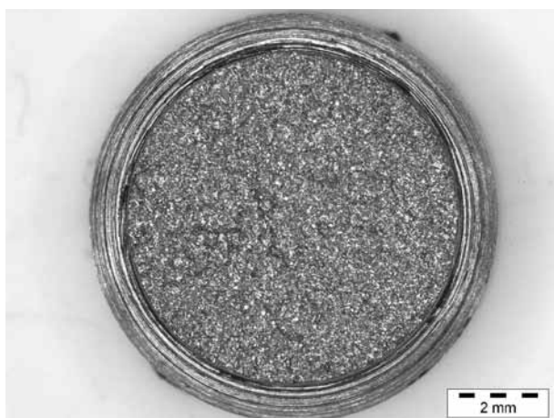
Figure 5: Fracture surface of a notched tensile specimen of steel quenched in water from 1250 °C. Microstructure: coarse-grained martensite
