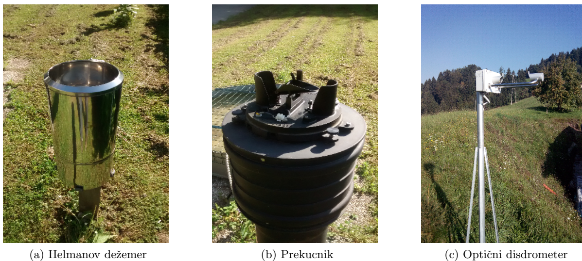
Slika 2.5: Prikaz merske opreme za točkovne meritve padavin (foto: Nejc Bezak) Figure 2.5: Measuring equipment for the precipitation measurements at specific point (photo: Nejc Bezak)
