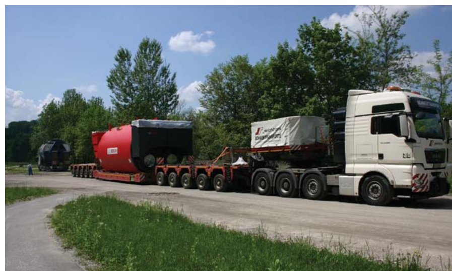
Izredni transport - samo prikolica je bila dolga 45m. Special transport - extension itself is 45 m long.
