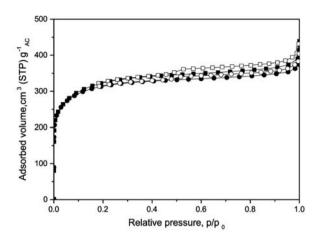
**Figure 1.** Adsorption isotherms of nitrogen obtained at -196 °C on the parent AC ( $\blacksquare$  – adsorption,  $\square$  – desorption) and the CsOH loaded ( $\bullet$  – adsorption, O – desorption) samples. Only the parent and the CsOH loaded samples are shown in figure, because all impregnated samples give nearly the same isotherms.
