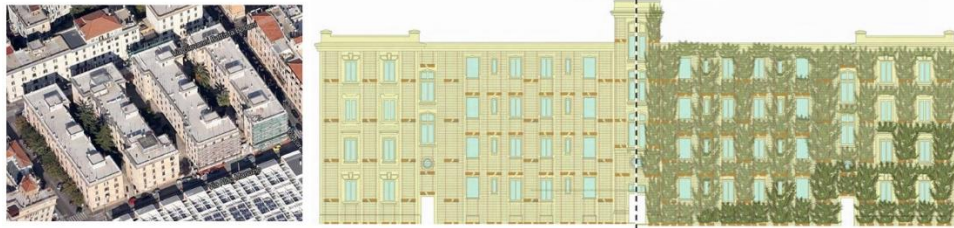
Figure 1: The picture of the case study block and the proposal for one of the courtyard façades. The bearing structure and the partition of the green wall: evergreen and deciduous plants in the lower and upper parts.
