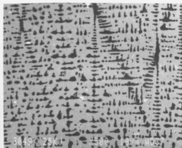
Slika 2: Mikrostruktura Sm-Fe-Ta litine z 2 at.% Ta, ki prikazuje \text{Sm}_2\text{Fe}_{17} fazo (sivo), dendrite primarnega železa (črno) in \text{SmFe}_2 fazo (belo). Figure 2: An SEM micrograph (SE/BSE Comp. Image) of the cast Sm-Fe-Ta alloy with 2 at.% of Ta showing \text{Sm}_2\text{Fe}_{17} (grey), Fe (dark), and \text{SmFe}_2 (white) phases.
