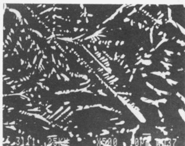
Slika 3: Mikrostruktura Sm-Fe-Ta litine s 5 at.% Ta, ki prikazuje \text{Sm}_2\text{Fe}_{17} (sivo) in \text{TaFe}_2 (belo) fazo. Figure 3: An SEM micrograph (SE/BSE Comp. Image) of the cast Sm-Fe-Ta alloy with 5 at.% of Ta showing \text{Sm}_2\text{Fe}_{17} (grey) and \text{TaFe}_2 (white) phases.
