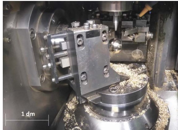
Fig. 1 Experimental setup for diamond fine turning of CuZn40Pb2
