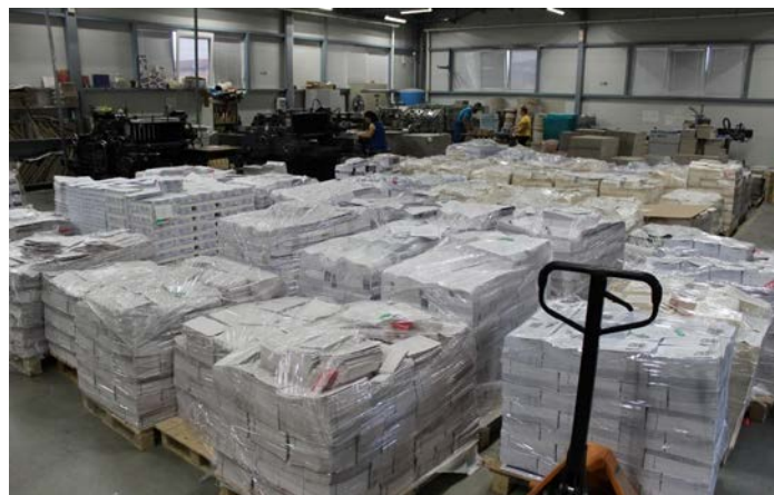
Fig. 2 A typical temporary or intra-warehouse of a printing SME. After finishing one operation, the tabs are stacked on pallets until they are requested by a following manufacturing process
