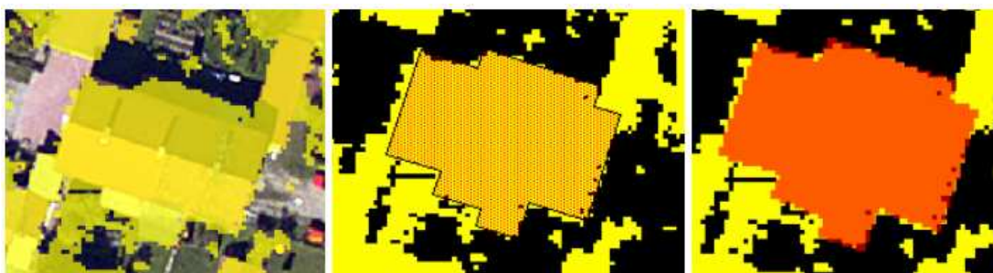
Slika 47: Podoba objektov z višino nad 1 m (rumeno) ter primerjava teh objektov z vektorizirano streho in rasteriziranim poligonom. Fig. 47: Raster image of objects, higher than 1 m (yellow) and comparison with vectorized and rasterized roof.
