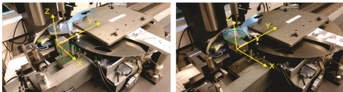
Fig. 6 Alignment of optics, camera and the moving table with fixed line scale
