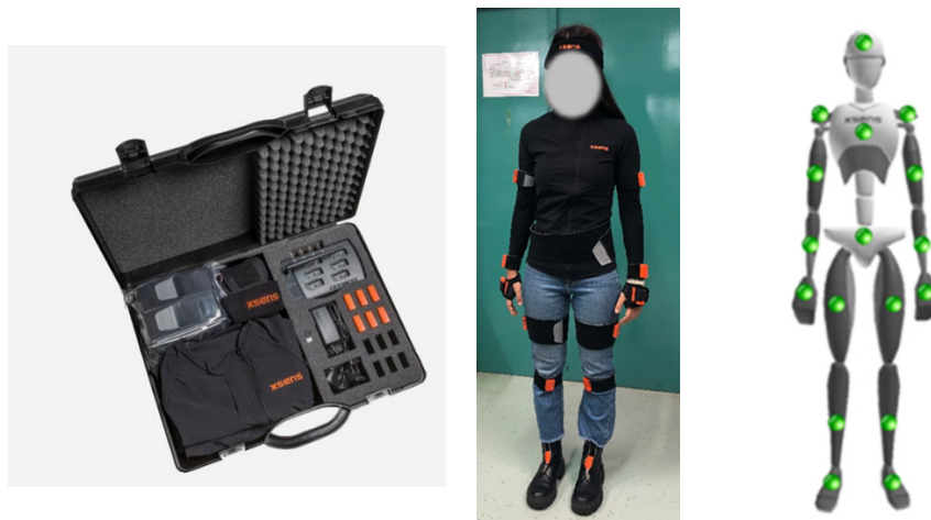
Fig. 2 Xsens MVN Awinda system for body movement data gathering and Xsens suit with sensors
