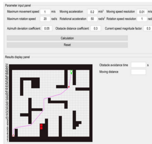
Fig. 2 Global path dynamic obstacle avoidance parameter test software setting interface
