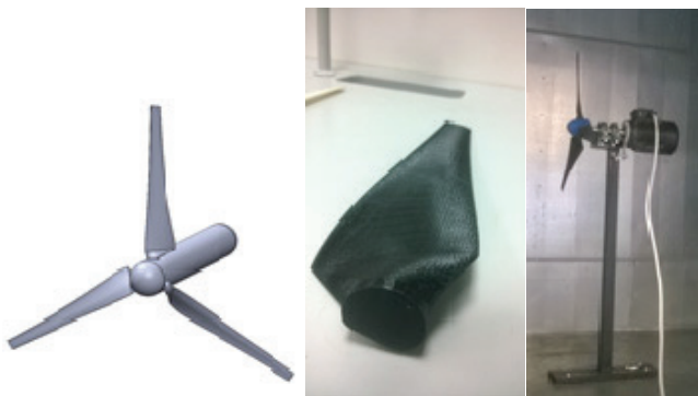
Figure 4: Wind turbine CAD model, blade 3D print and turbine measurements in wind tunnel
