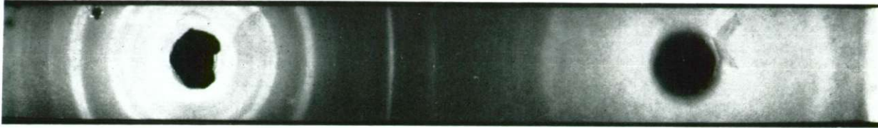
1. sl. Debeygram stragarskega azbesta z jalovino (Stragari 4 K, kobaltova anoda) Fig. 1. X-rays diffraction pattern of the Stragari-asbestos with the waste (Spec. Stragari 4 K, Co anticathode)
