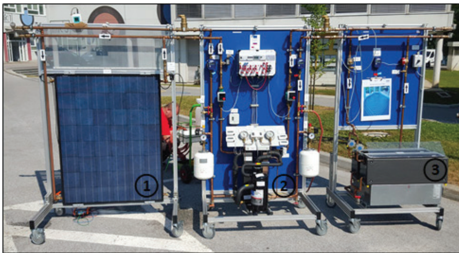
Figure 4: PV/T system of a German manufacturer WIOSUN: 1. Silicon poly-crystalline PV/T water module, 2. heat pump (evaporator/compressor/condenser), 3. Convector, [23].
