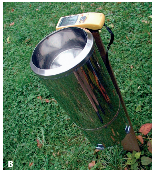
Slika 2a) Ombrograf Onset RG2-M in b) Helmanov dežemer za merjenje padavin na prostem Figure 2a: Onset RG2-M and b) Helman rain gauge for measuring gross precipitation.
