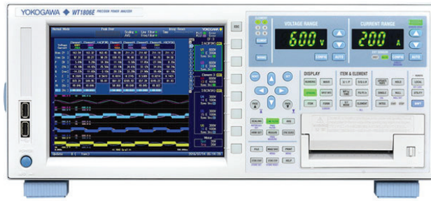
Figure 8: Power analyser Yokogawa WT1806
