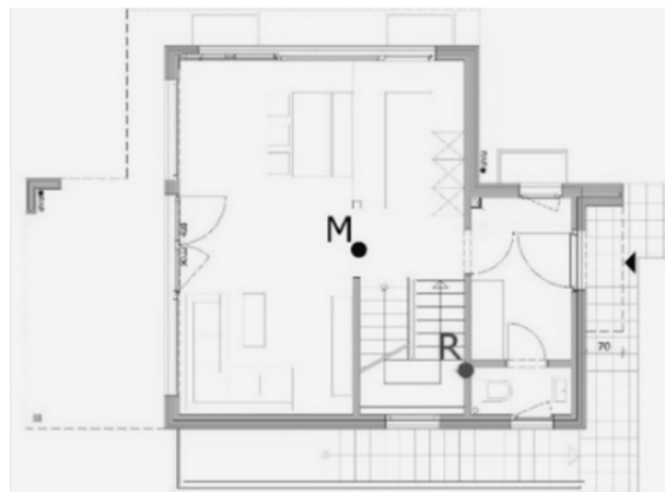
Fig. 2 Phenomenon of torsion on the floor due to deviation of mass (M), and centre of stiffness (R), randomly chosen case
