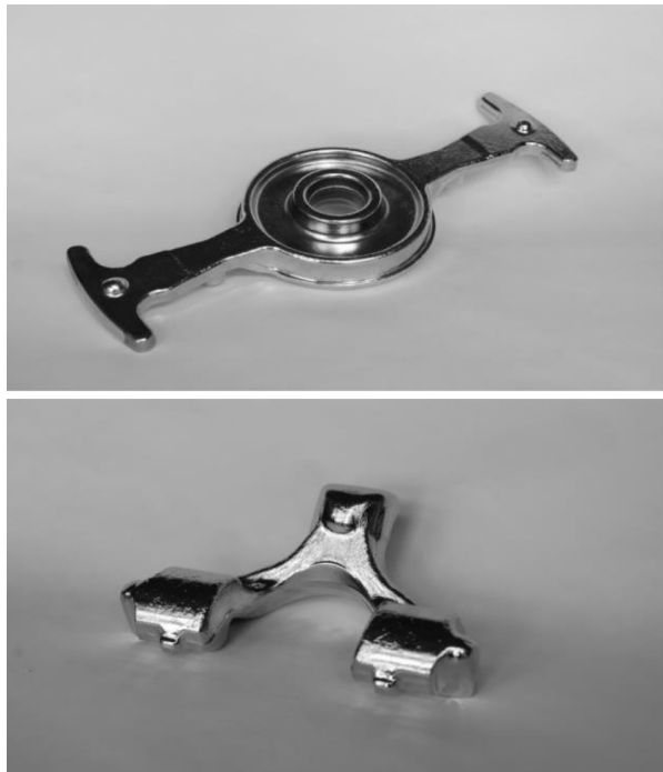
Figure 4: Demonstration products: AHSS steels forgings heat-treated using the Q&P process
