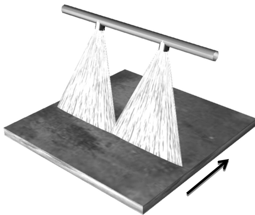
Figure 4: Visualization of the nozzle configuration with the 0° twist angle. The spray width of each nozzle is 49 mm and the overlap is 6 mm. The arrow indicates the plate movement direction.
