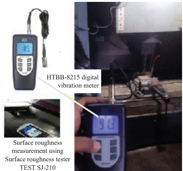
Fig. 3. Measuring devices: vibration meter and surface tester SJ-210
