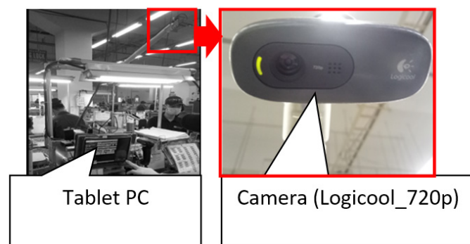
Fig. 10 Actual camera system in process
