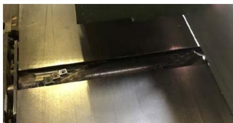
Figure 2. Cutter head with segment knives
