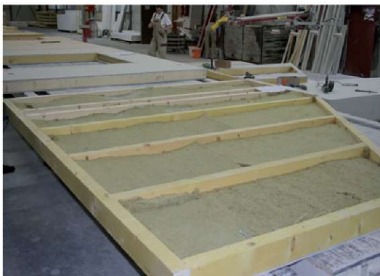
Figure 1: Composition of a timber-frame wall element; a.) macro-panel system, b.) single wall element
