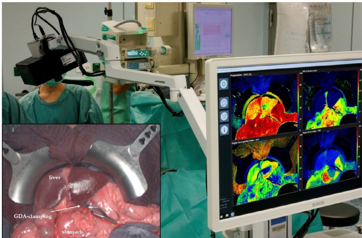
FIGURE 6. Hyperspectral imaging (HSI) acquisition system in the operating room. Hyperspectral images were acquired within a few seconds with physiologic HSI parameters displayed in false colors.
