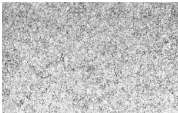
Figure 5: 100x, Microstructure of the steel 4. Tempered martensite, acicular ferrite and cementite precipitates Slika 5: 100x, Mikrostruktura jekla 4. Popuščeni martensit, acikularni ferit in cementitni izločki
