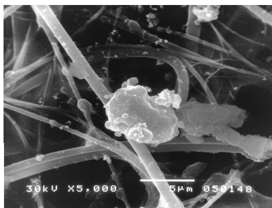
Figure 4. Coarse Fe-rich particle from the PM_{2.5} sample, November 2003 and X-ray microanalysis spectra
