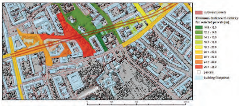
Figure 5. Spatial analysis of the minimum depth to the subway tunnel, performed for parcels where the subway tunnels are located; Source: with the use of data from "Metro Warszawskie Sp. z o.o." and ALS data from Head Office of Geodesy and Cartography.
