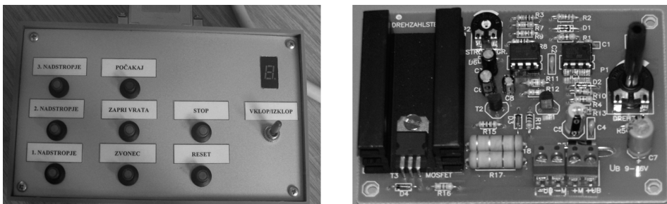
Fig. 2: Operating panel in the lift car
