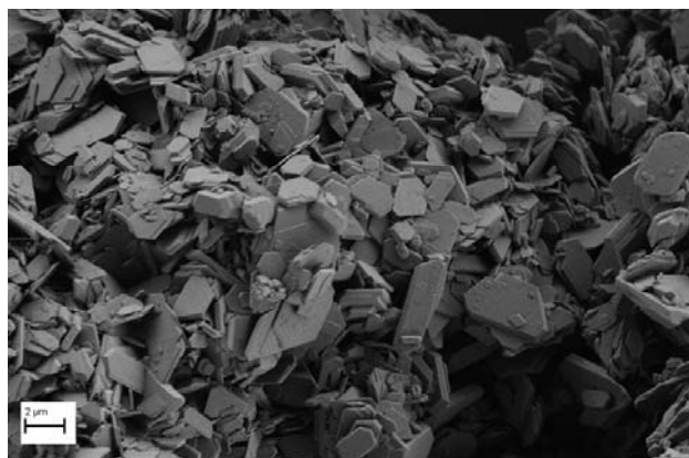
Figure 10. SEM picture of a boehmite-based monocarbonate (24 h; with calcite 4.2).
