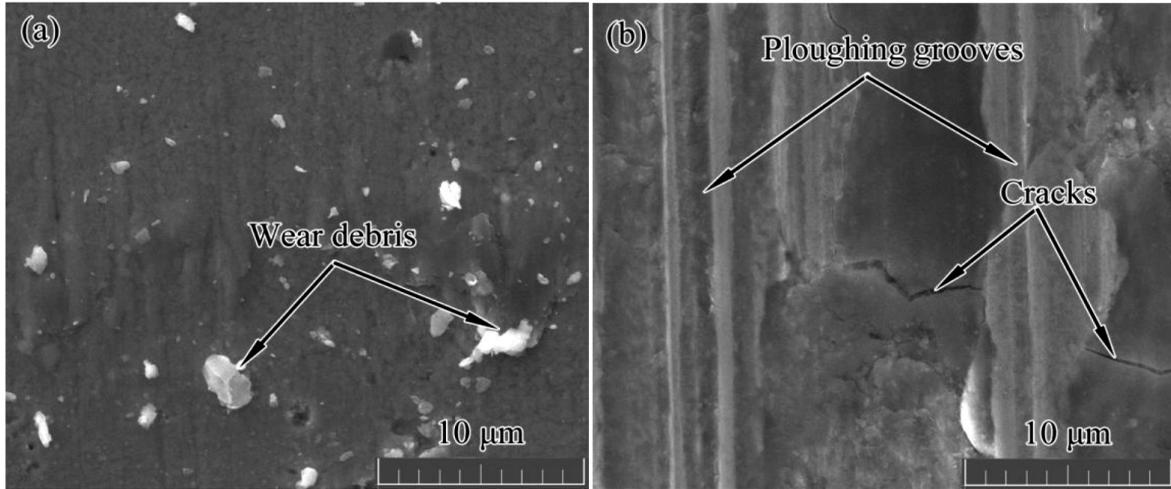
**Figure 6:** Worn surface morphologies of the Ta coating and CrNi3MoVA steel
