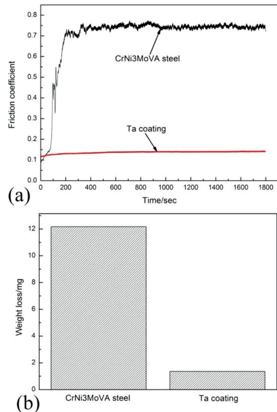
**Figure 5:** Friction coefficient and wear mass of the Ta coating and CrNi3MoVA steel
