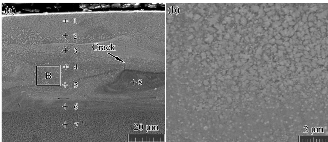
**Figure 3:** a) Cross-section and b) magnification of region B of the as-deposited Ta coating
