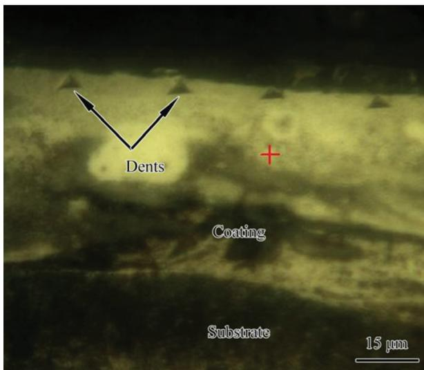
**Figure 1:** Indentation positions of the hardness and elasticity modulus test on the cross-section of Ta coating
