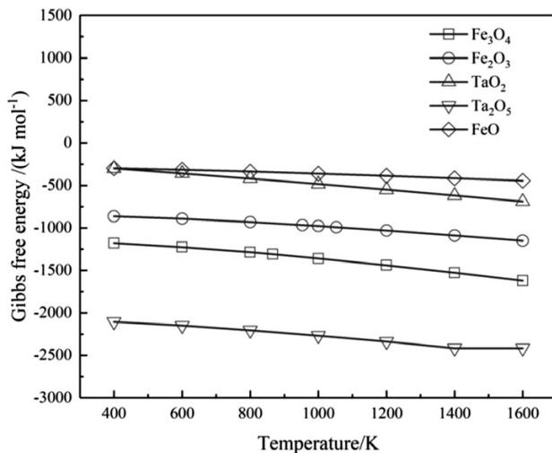
**Figure 7:** Gibbs free energy change in the oxides of Ta and Fe at various temperatures
