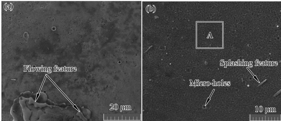
**Figure 2:** a) Surface morphology at low magnification and b) high magnification of the as-deposited Ta coating
