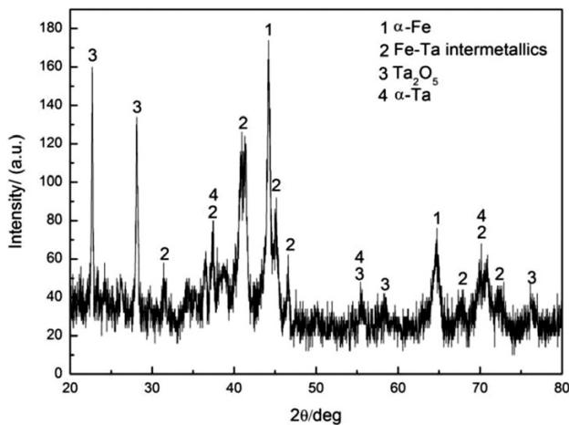
**Figure 4:** XRD pattern of the as-deposited Ta coating
