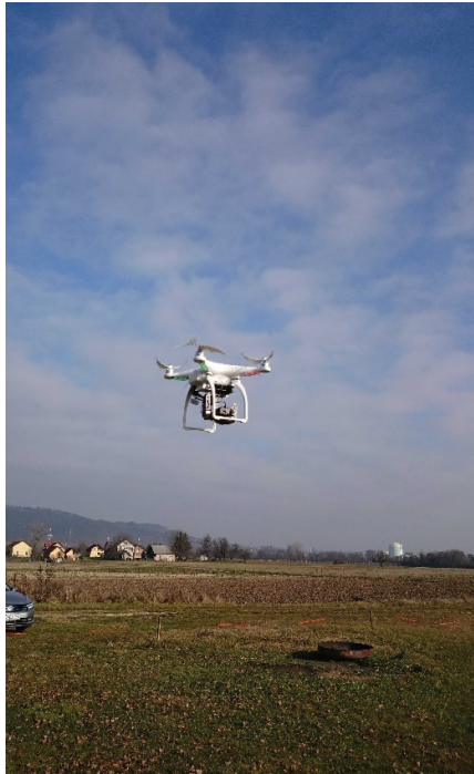
Figure 6: Thermovisional inspections using drones
