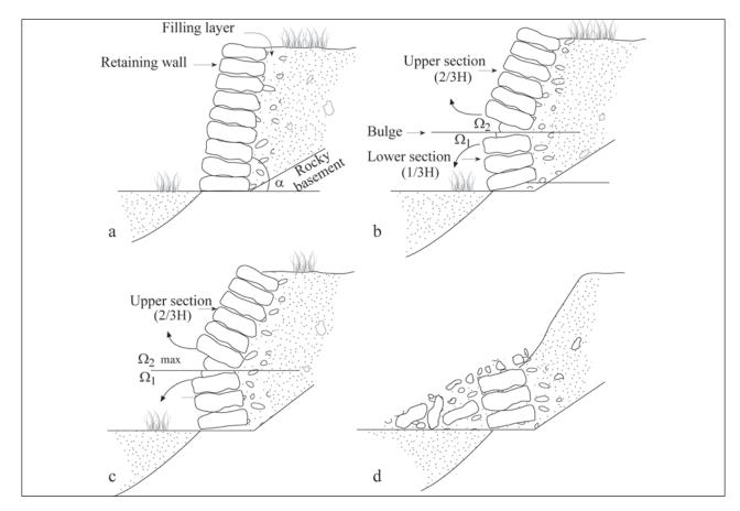
Figure 9: Stages in the process of wall collapse: a) retaining wall; b) bulge on the 1/3 lower section; c) bulge collapse; d) wall collapse.
