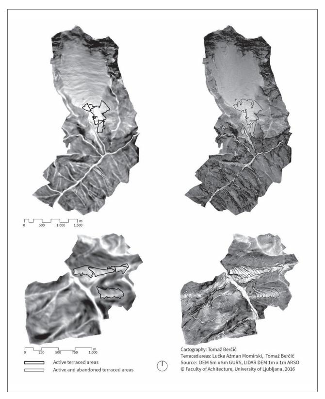
Figure 4: The top left image shows DEM5 slope data with an active terrace overlay for the settlement of Rut. The top right image shows LIDAR data with detected active and abandoned terraced areas for the same pilot area. The bottom left image shows the DEM5 slope data with an active terrace overlay for the settlement of Smoleva. The bottom right image shows LIDAR data with detected active and abandoned terraced areas for the same pilot area.
