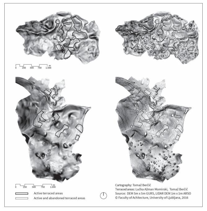
Figure 6: The top left image shows the DEM5 slope data with the active terrace overlay for the settlement of Dečja Vas. The top right image shows LIDAR data with detected active and abandoned terraced areas for the same pilot area. The bottom left image shows the DEM5 slope data with the active terrace overlay for the settlement of Merče. The bottom right image shows LIDAR data with detected active and abandoned terraced areas for the same pilot area.
