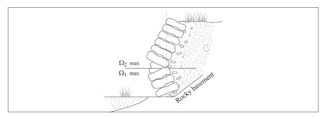
Figure 8: Wall bulge on the 1/3 lower section.
