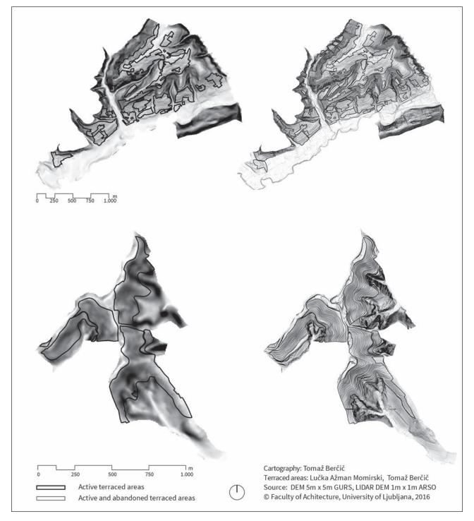
Figure 7: The top left image shows the DEM5 slope data with the active terrace overlay for the settlement of Krkavče. The top right image shows LIDAR data with detected active and abandoned terraced areas for the same pilot area. The bottom left image shows the DEM5 slope data with the active terrace overlay for the settlement of Jeruzalem. The bottom right image shows LIDAR data with detected active and abandoned terraced areas for the same pilot area.
