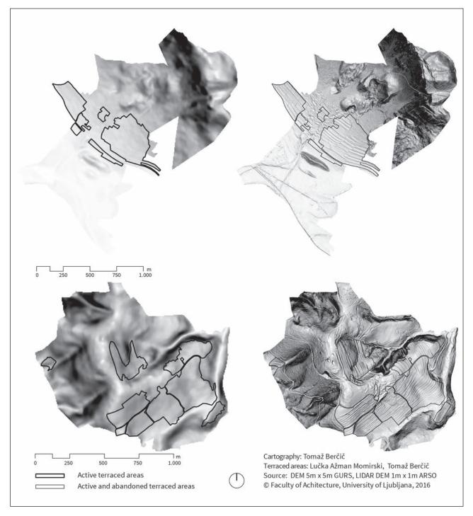
Figure 5: The top left image shows the DEM5 slope data with the active terrace overlay for the settlement of Rodine. The top right image shows LIDAR data with detected active and abandoned terraced areas for the same pilot area. The bottom left image shows the DEM5 slope data with the active terrace overlay for the settlement of Velika Slevica. The bottom right image shows LIDAR data with detected active and abandoned terraced areas for the same pilot area.
