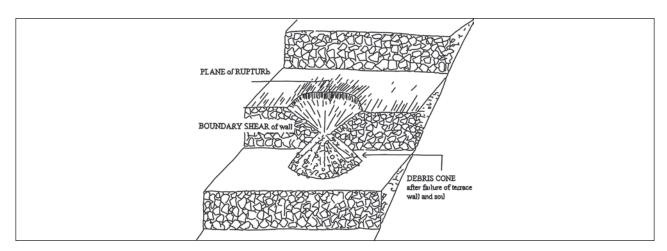
Figure 12: Schematic view of a collapsed terrace.
