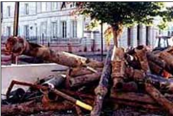
Figure 1. Corrosive damage to pipe lines.
