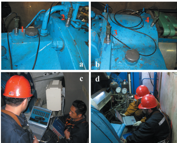
Fig. 1. Test system on field wind turbine gearbox; a) two transducers in the front of the gearbox, b) two transducers in the rear of the gearbox, c) data acquisition system, d) data analysis and processing
